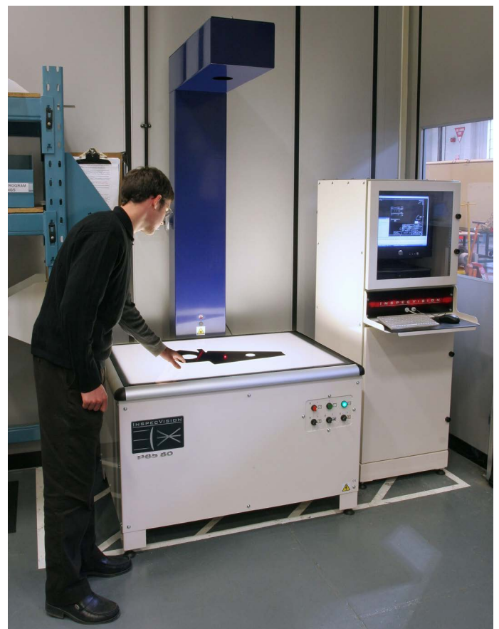
Figure 1: Marshall Aerospace using their P65.50 to measure aircraft components. The machine is pictured in their inspection department but will be moved to the shop floor.
