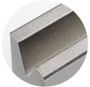
Left: Dies coated with LASERdur ZN keep the galvanized zinc layer intact.
