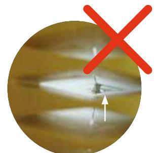
If there are any adhesive residues on the filter fleece, both the filter's performance and its service life will be reduced.
