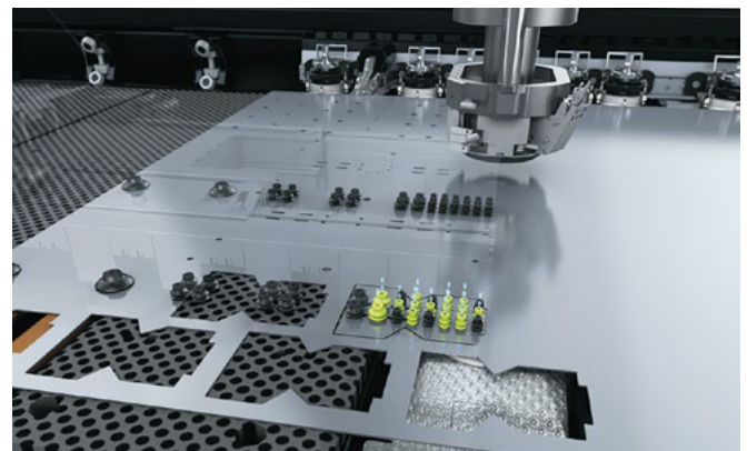
Suction cup slats with individually activated suction cups.
