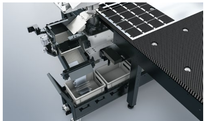
Good parts enter an intermediate buffer via a part chute.
