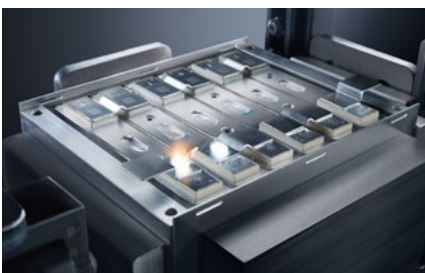
Welding of aluminum battery cases.
