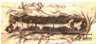
Welding of battery foil stacks consisting of 100 copper foils with TruDisk 2021. Left: Regular seam surface without ejections. Right: Cross-section of the poreless weld seam with large joint area.
