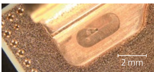
Welding of copper contacts on DCB substrate with well controlled welding depth using TruDisk 1020.
