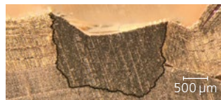
Welding of battery foil stacks consisting of 100 copper foils with TruDisk 2021. Left: Regular seam surface without ejections. Right: Cross-section of the poreless weld seam with large joint area.
