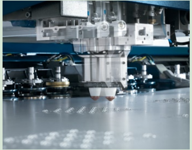
The laser can move in two directions on auxiliary axes.
