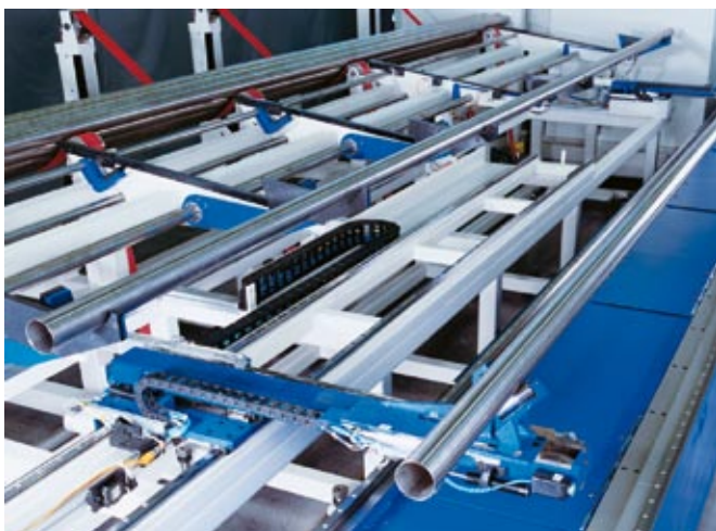
Automatic separation of round tubes.
