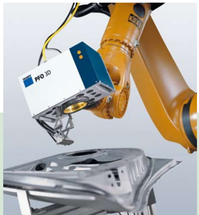
Programmable focusing optics PFO 3D.
