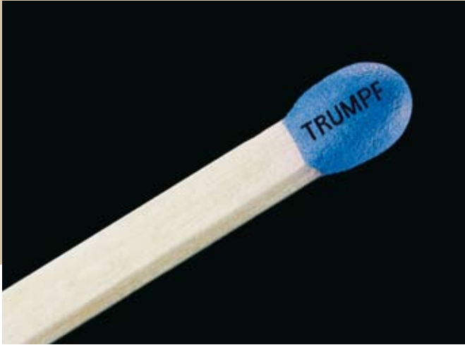
Cold processing with picosecond pulses on a match-head.
