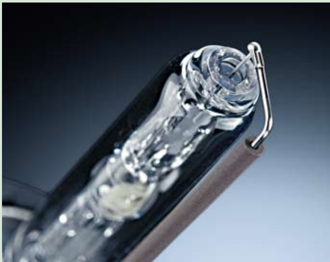
Filigree spot welds.
