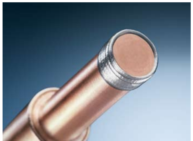
Laser deposition welding on beryllium-copper.
