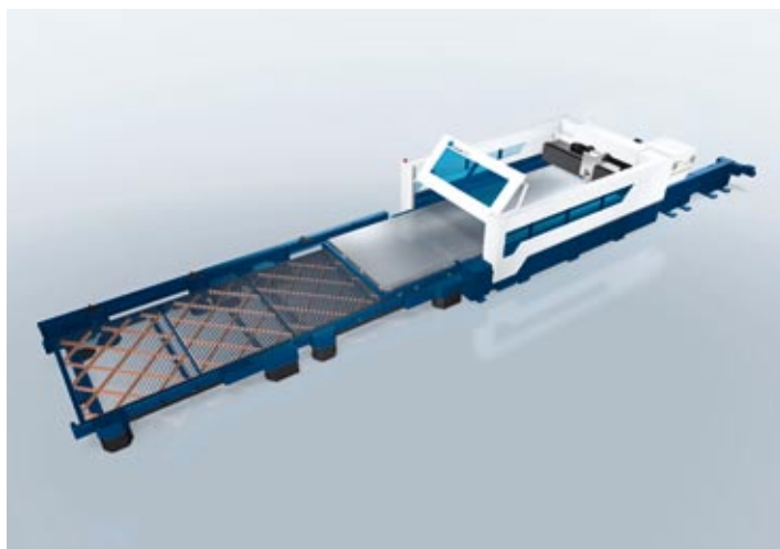
Highly productive with an oversized format pallet changer.
