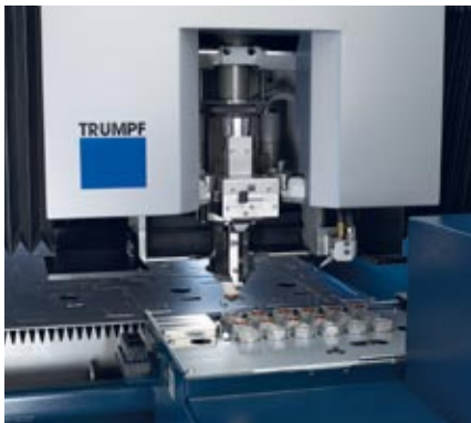
The optional nozzle changer switches nozzles automatically.
