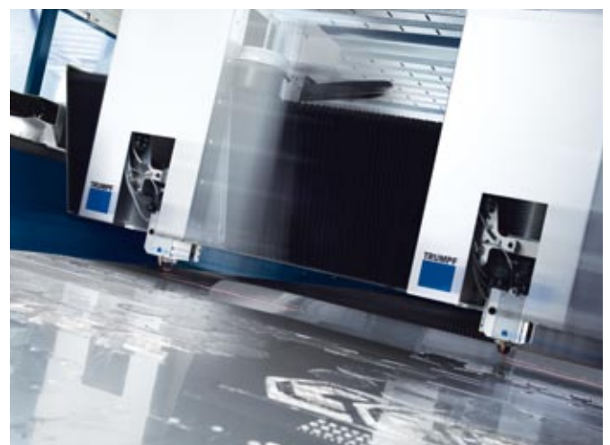
Twice the productivity with two cutting heads.
