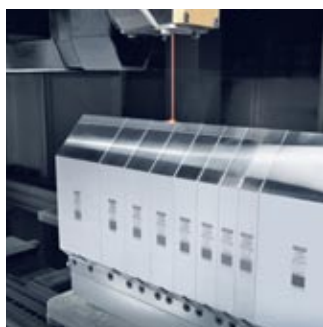
The LASERdur process used to harden the tools.
