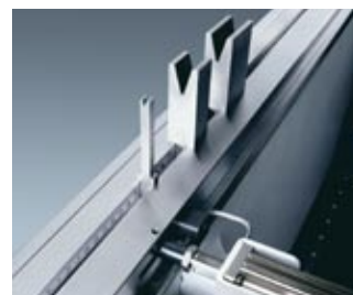
Lower tool holder system for the TruBend Series 5000.
