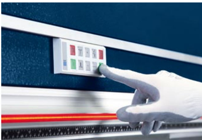
Mobile Control enables the operator to control machine functions remotely, without having to move from place to place.
