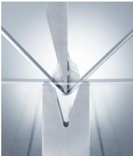
Automatic bending with angle sensor ACB.
