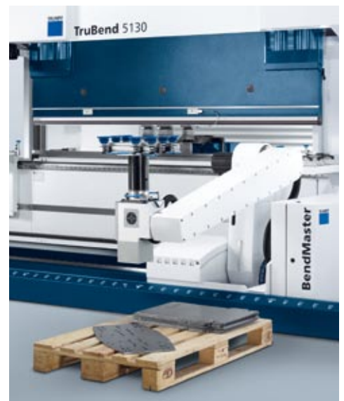
BendMaster (60) collecting fine positioning data.
