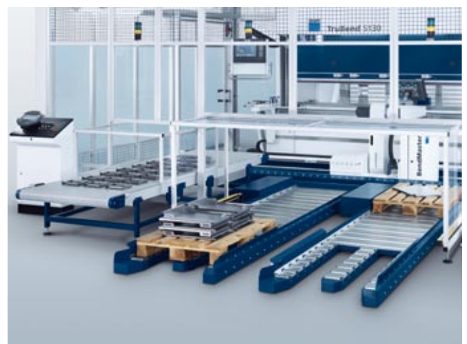
Conveyor belt and pallet feeder.
