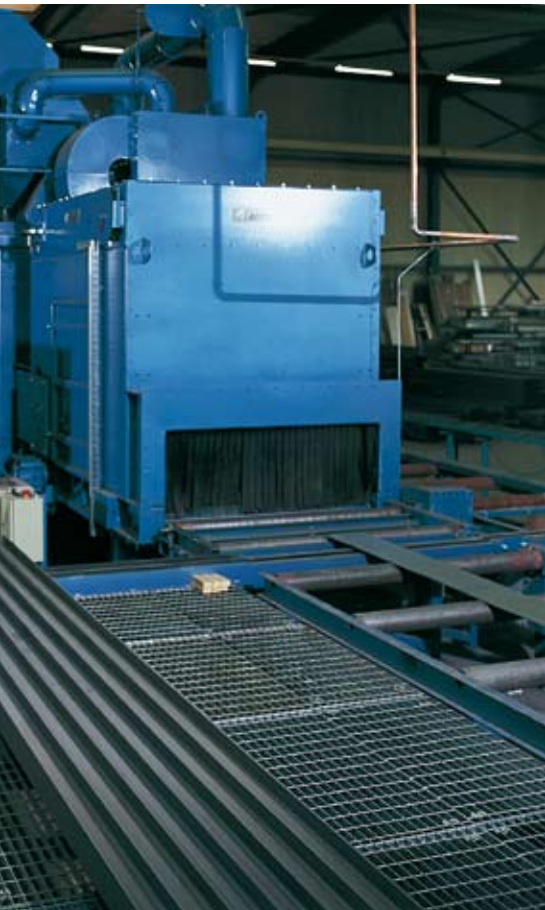
Roller conveyor blast machine with crossover conveyor technology.
