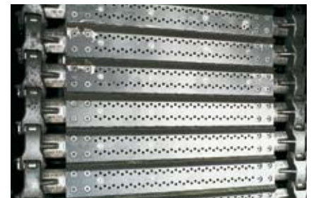
Configuration of steel mill tumble blast machines with new wear-parts.
