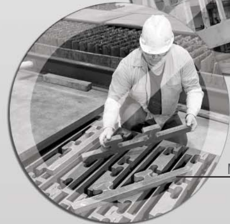
PROBLEM 5: REMOVAL OF SKELETON Labor Intensive, Creates Scrap, Safety Concerns
