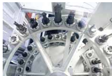
Maintenance free disc magazine
