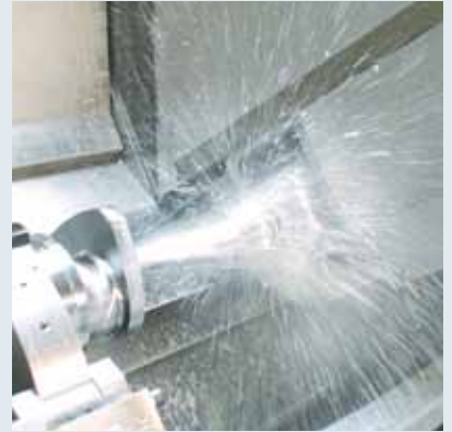
80 bar coolant pressure
