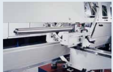
Production time parallel loading for boring bars
